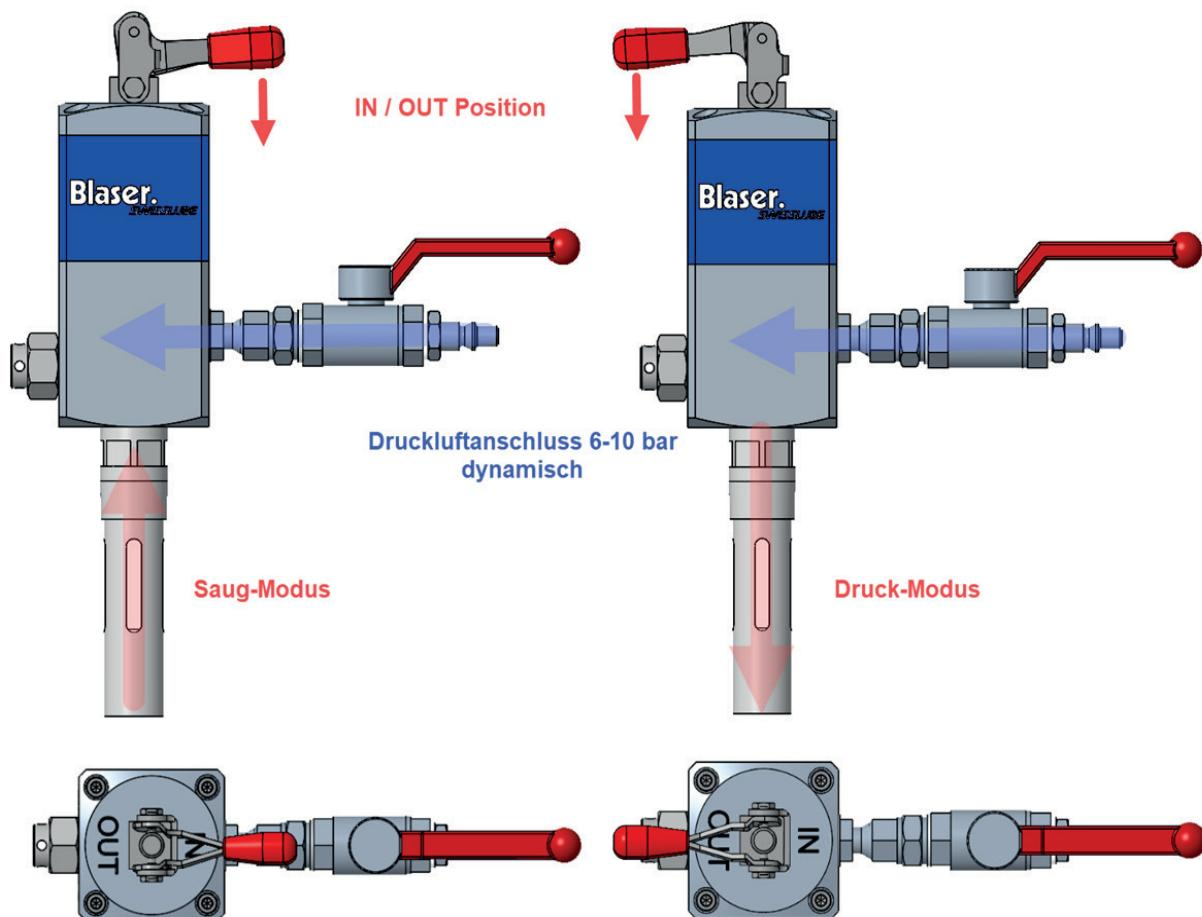
Druckluftanschluss 6-10 bar dynamisch = compressed air connection (6-10 bar dynamic) / Saug-Modus = Suction mode / Druck-Modus = Pressure mode
