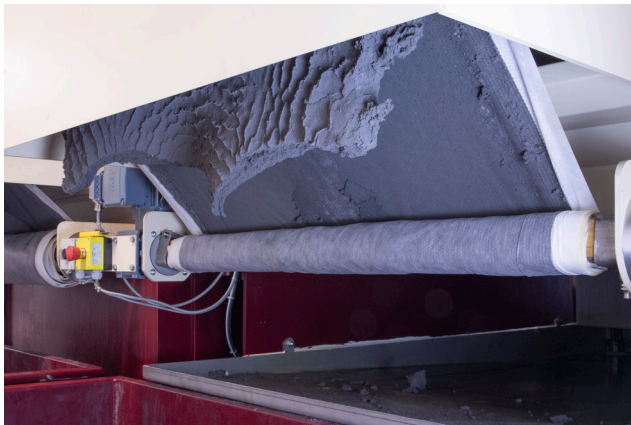
Compact filter cake thanks to the excellent filterability
