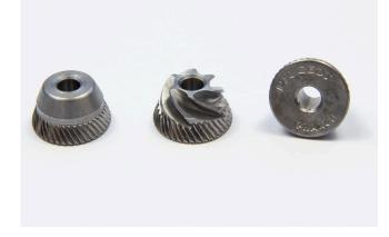
PSP Peugeot had heard of the Liquid Tool by Blaser Swisslube. The ability to achieve a measurable added value thanks to the optimum metalworking fluid evoked their interest. They wanted to improve the cycle and tool life in the demanding machining process of gear hobbing, in which the "poire" (pear), made of stainless steel S250, is ground.
